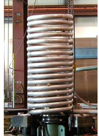
↑ 28" dia. x 120" long pipe coils
