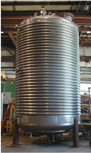
↑ Tank Dimensions: 134" dia. x 418" (incl. legs) Tank Weight: 68,200 pounds
