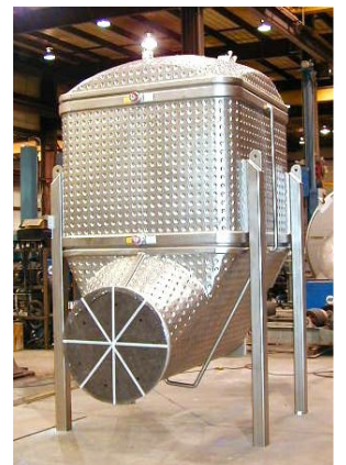
Surge Tank Hopper →
