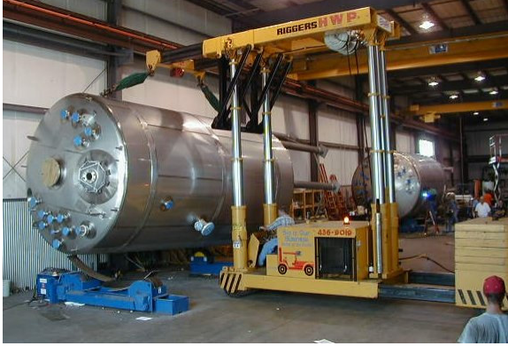
↑ Tank Dimensions: 134" dia. x 418" (incl. legs) Tank Weight: 68,200 pounds
