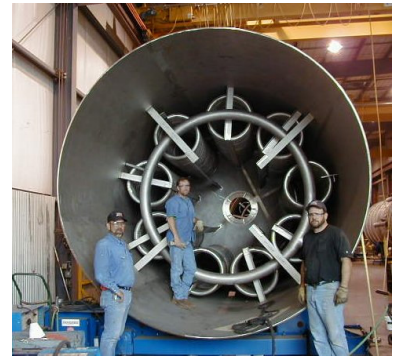
↑ (9) full-pipe coils in tank weighing a total of 20,300#
